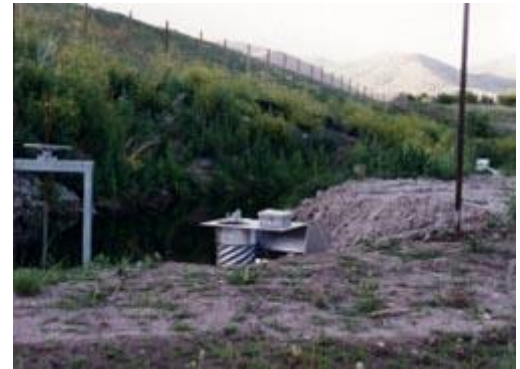
Mantua Wetlands, 2 ft. rectangular weir, custom stilling well, instrumented with a FP10C Float and Pulley attached to a CR10X Data logger.
