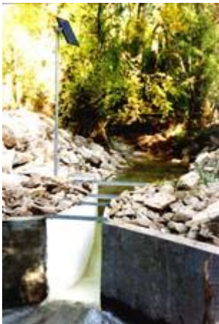
Box Elder Creek, 9" FRP Parshall Flume with attached 12" stilling well, instrumented with PT1830 DRUCK pressure transducer attached to a CR510 Data logger.
