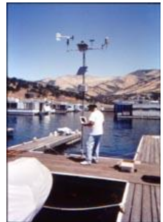
KRWCD personnel downloading data from the Pine Reservoir weather station located on the floating marina boat dock.
