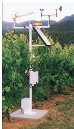
This vitaculture site in Australia integrates meteorological, soil, and crop measurements.
