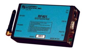
The RF401 shown above has a 15730 antenna that attaches directly to the radio. This omnidirectional antenna should reside inside a building or enclosure. It has a knuckle joint that can be oriented at right angles.
