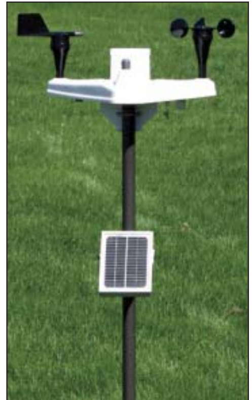
WeatherHawk provides real-time weather measurements and calculates ET_o on an hourly and daily basis.
