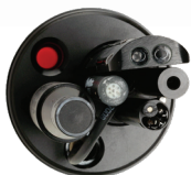
View of sensors on sub-4 in with turbidity, pressure, and RDO.
