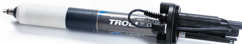
View of sensors on sub-2 in with pH, conductivity, and RDO.
