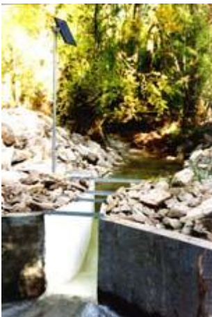
Box Elder Creek, 9" FRP Parshall Flume with attached 12" stilling well, instrumented with PT1830 DRUCK pressure transducer attached to a CR510 Data logger.
