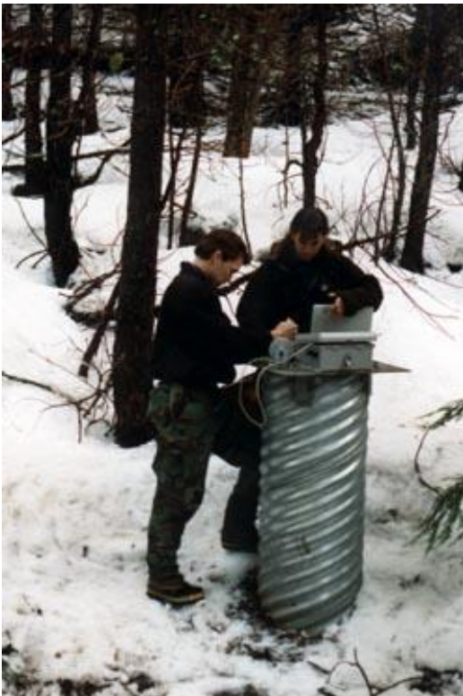
R2 Data logger with attached FP10C Float & Pulley Sensor being
