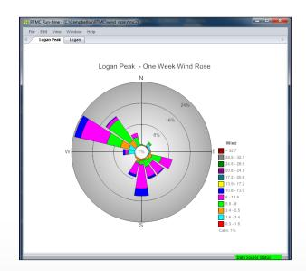
With RTMC Pro, users can create a wind rose report that displays the distribution of wind directions at various wind speeds.
